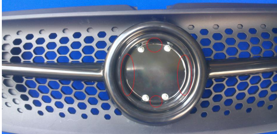
Photo 4: Put some Polyurethane glue at these four places.
