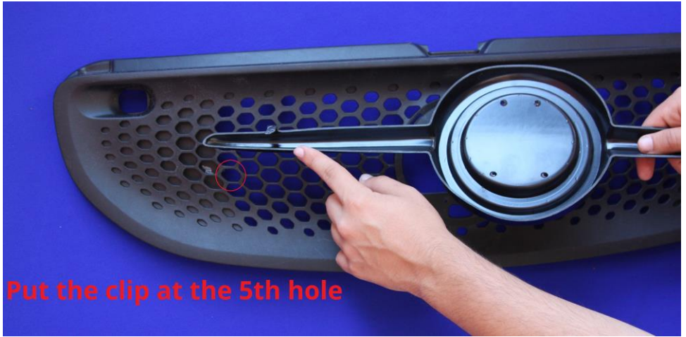
Photo 2: These are the clips from the back side of the Smart Power Design's Front Grille.
