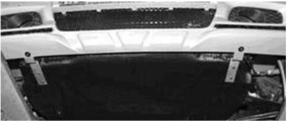
Photo 6: Stabilizing the Front Spoiler with the metal brackets
