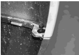
Photo 12: Expansion bolts on the rear spoiler
