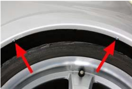
Photo 3: Positions two of the four screws
