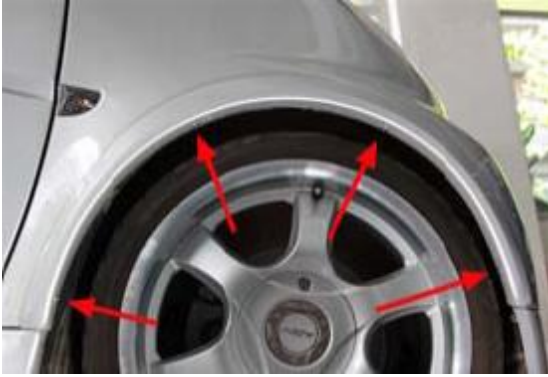
Photo 2: Positions of the screws, there are four on each Fender Flare
