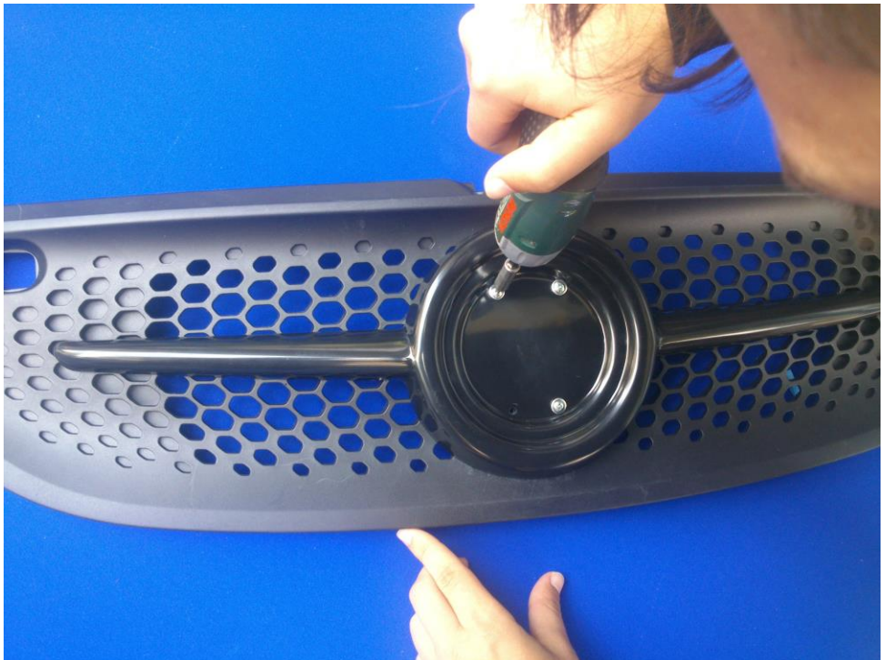
Photo 3: Screw the 4 screws.
