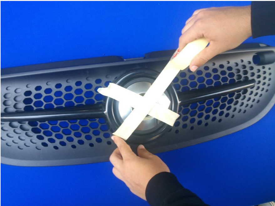
Photo 5: Place the Emblem you have received and stick it to the center with the adhesive tape.
