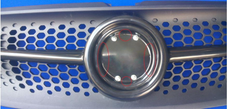
Photo 4: Put some Polyurethane glue at these four places.
